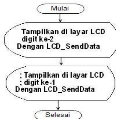
Gambar 10. Flowchart Sub Program Tulis_BCD .
