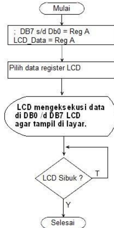
Gambar 7. Flowchart Sub Program LCD_SendData .
